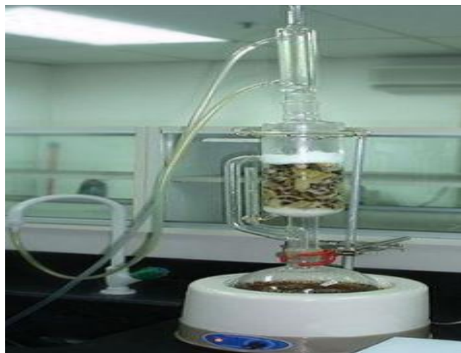
Figure 1: Soxhlet extraction apparatus
