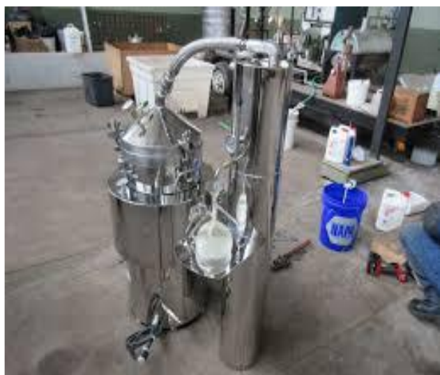
Figure 2: Hydro distillation apparatus
