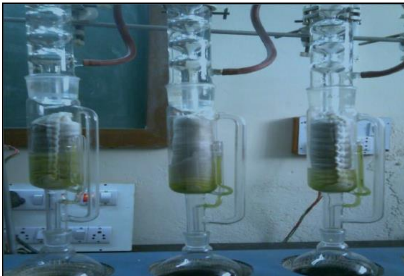
Fig. 2: Extraction using Soxhlet apparatus assembly
